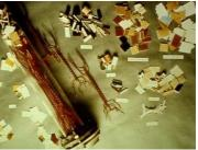
Long Term Thermal Aging (LTTA) testing is designed to monitor degradation of the insulation system. It involves the proposed EIS at three or more elevated temperatures with intermittent dielectric proof testing. After each heat cycle, samples are also subjected to repeated series of environmental exposures, such as mechanical stress, cold shock, and humidity. The performance of the proposed (candidate) EIS is compared to a control EIS with previously established rating.
